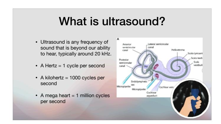
Again, a hertz is one cycle per second, a kilohertz is 1000 cycles per second, and a megahertz equals 1 million cycles per second
